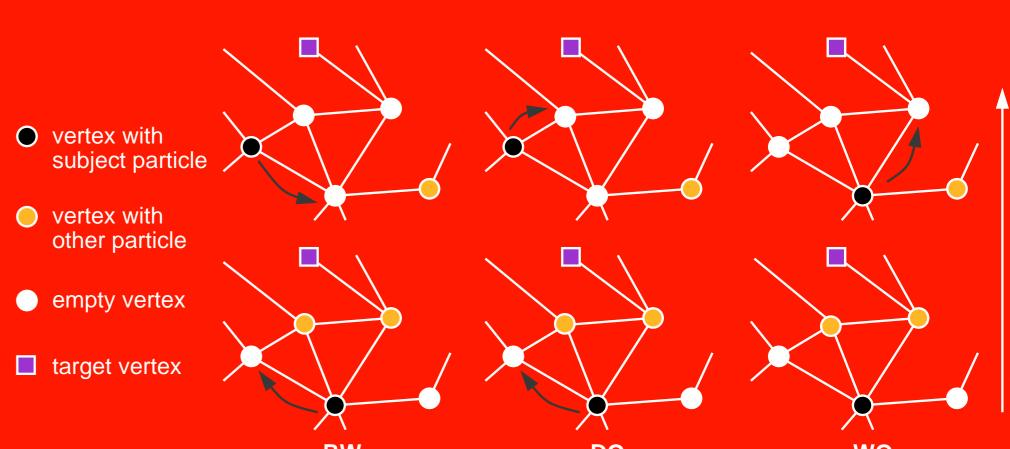
Wait at Obstacle (WO): Like DO but if no vertex closer to the target is free, then the particle waits.
